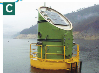
C Automatic water quality monitoring equipment, known as Takenoko (bamboo shoot)
